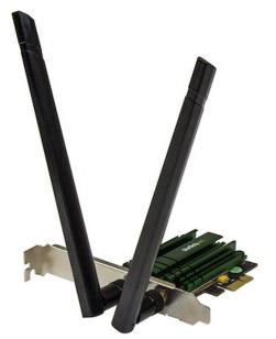
The PEX867WAC22 PCI Express AC1200 Wireless Network Adapter lets you add dual-band Wireless-AC connectivity to a desktop computer through a PCIe slot.
